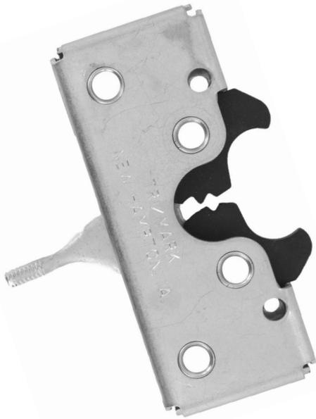
This two rotor latch is a sub-platform to the TriMark proven 050-0100 series latch and is designed for medium to heavy-duty applications for on or off-highway entrance doors, compartments and access panels. It features an internal trip mechanism for applications where it is desirable to have the release mechanism inline with the latch and a single position latch.
